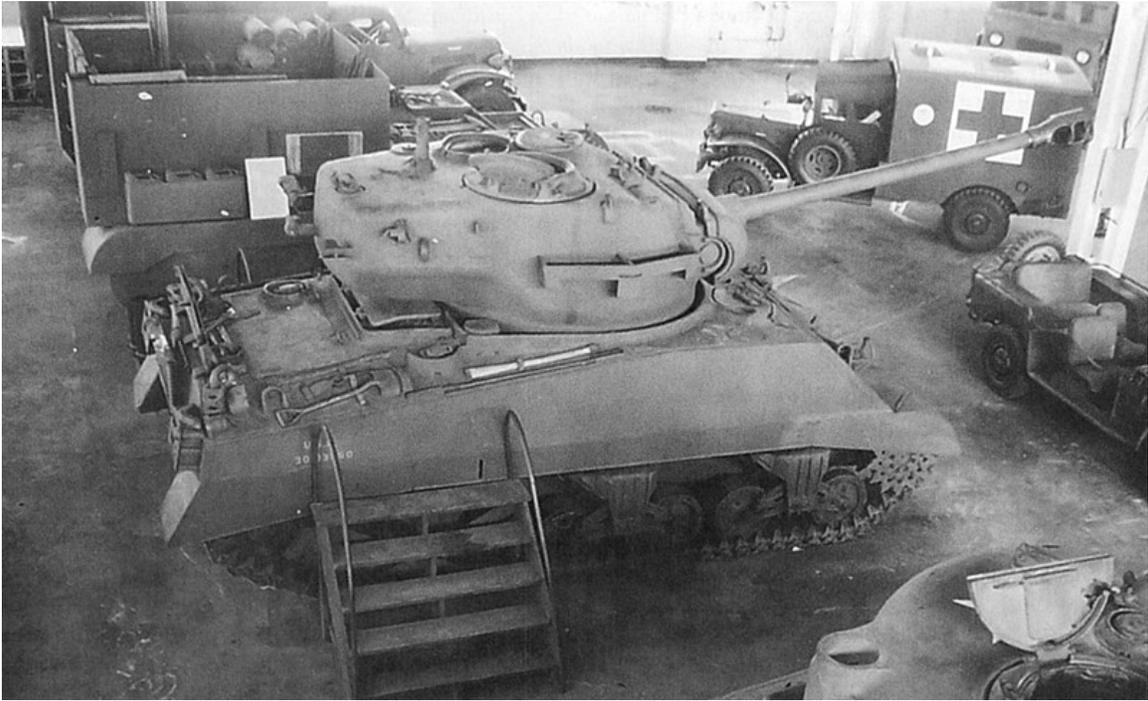
M4 with T-26 turret and 90mm cannon at Detroit Tank Arsenal. Instead of shipping M4s with 76mm guns, or M26s, this is what the Armor Branch was after.
